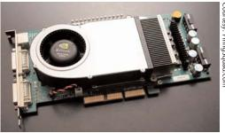
The GeForce 6800 Ultra. Note the large heatsink and fan combination, and the two DVI connectors
